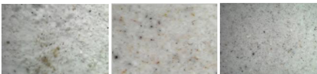
Fig. 2 The surface of a washed kaolin sample at the beginning; after cycles 35; and after 50 cycles (from left to right)
