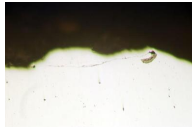
Figure 9 Crack beneath the surface x100 (on the left side of the macro crack)
