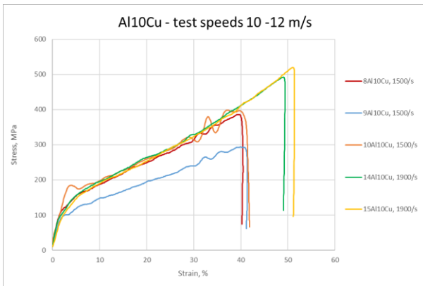
Fig. 3 SHPB dynamic test results at 10-12 m/s
