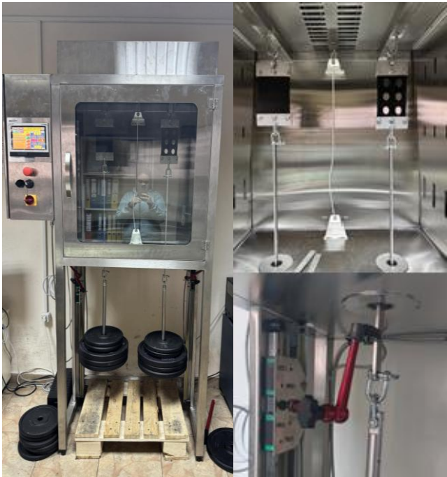
Fig.1 Universal creep testing stand
