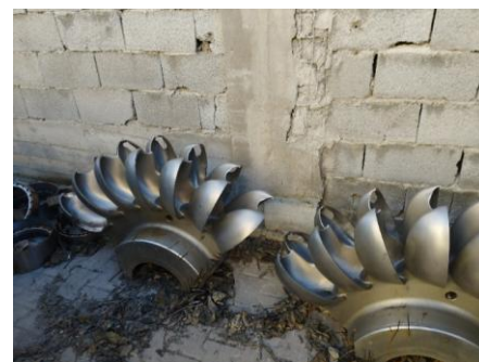
Figure 2 Cut turbine wheel halves with a buckets
