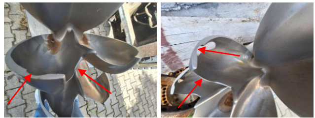
Figure 8 Erosion roll out of the bucket surface during exploitation
