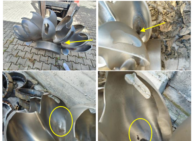
Figure 7 View of bucket from the inner side Pozitions where perforation starts
