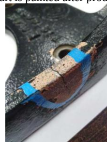
Figure 2 Crack on the specimen
