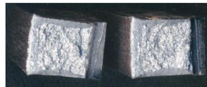
Figure 15 Fractured surface of impact specimen
