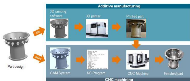
Fig. 9 General concept of technological integration of AM and cutting processes (source: Siemens)
