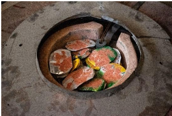
Fig.1. Disposition of the cans into the resistance furnace
