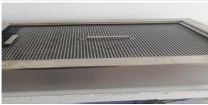
Fig. 4 The vent of the dryer
