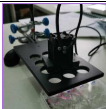
Fig. 2. A single 808 nm near-infrared light (NIR) laser system used for irradiation of cancer cells
