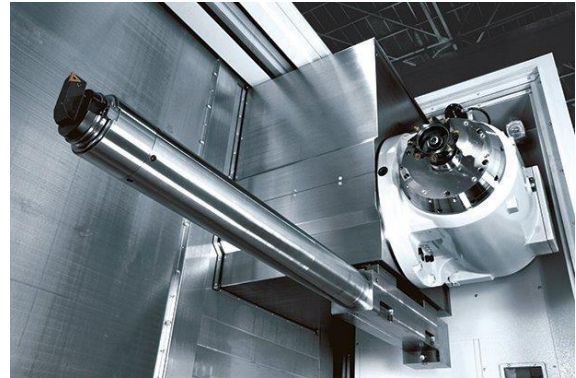
Fig. 6 Deep boring on multi-tasking machine tool (source: Yamazaki Mazak Co.)
