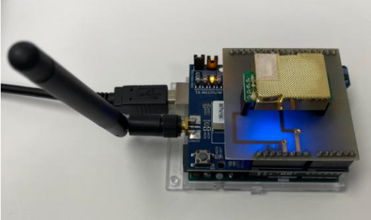
Fig. 3 Photograph of CO 2 sensor for an IoT system with Sigfox
