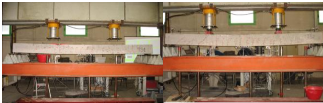
Fig. 6 Beam T1 & T2 - Concrete crushing failure, full cracked section ( \approx 90 kN)
