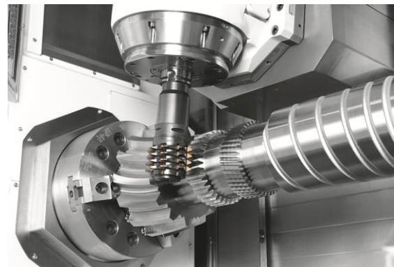
Fig. 8 Machine gears with multi-tasking machine tool (source: Yamazaki Mazak Co.)
