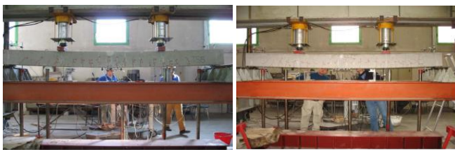
Fig. 7 Beam T3 ( \approx 102 kN) & T4 ( \approx 55 kN) - Concrete crushing failure, full cracked section
