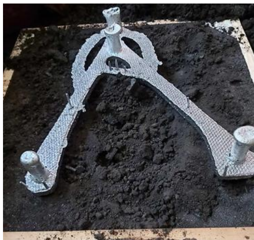
Fig. 6. The casting, after destruction of the sand-clay mold
