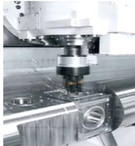
Fig. 7 Boring by U-axis tool (source: D'andrea TA-C160)
