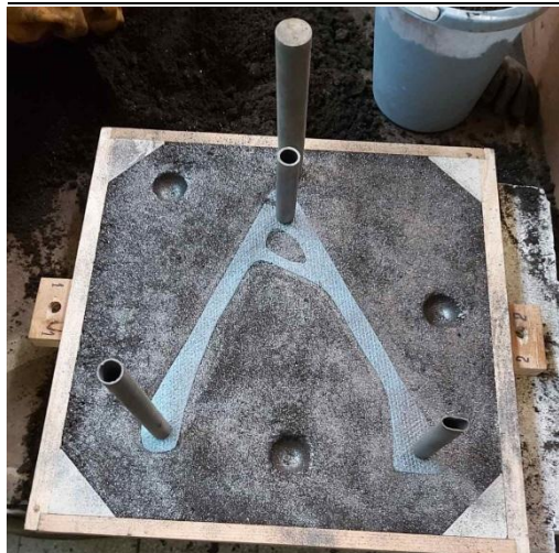
Fig. 5. Orientation of the sprue, feeders and overflows
