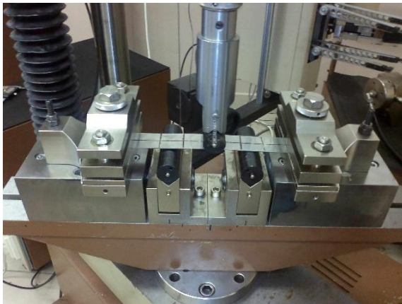
Fig. 5 Three-point bending test [10].
