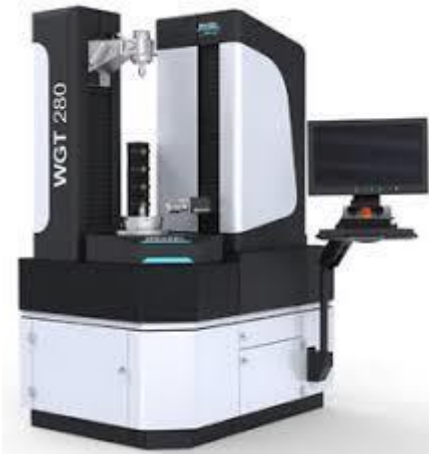
Fig. 3 3D measuring machine Wenzel WGT 280
