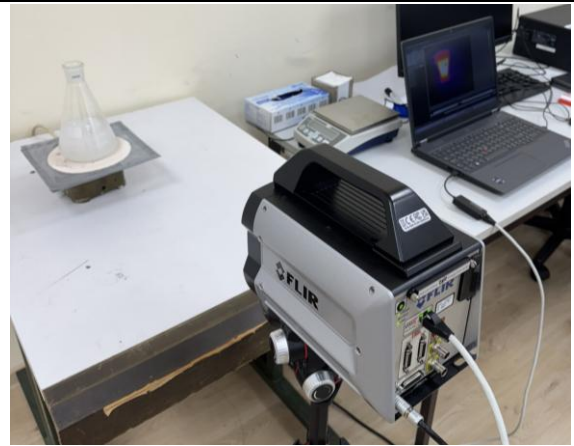
Fig 5: Thermographic imaging with FLIR X6800sc MWIR
