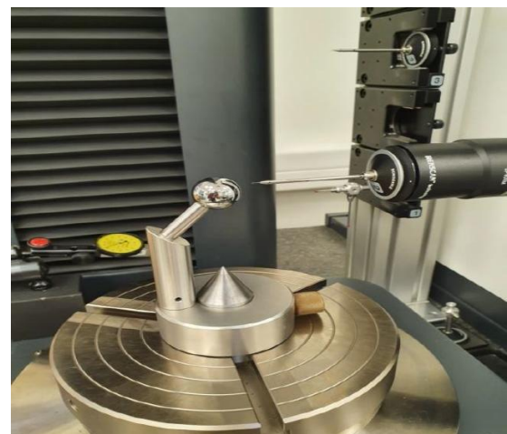
Fig. 4 Calibrating the measuring probe
