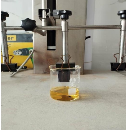
Fig. 1 Experimental setup for layer deposition using the immersion method
