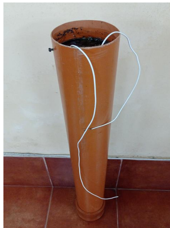
Fig. 2 Photo of single segment of the composter
